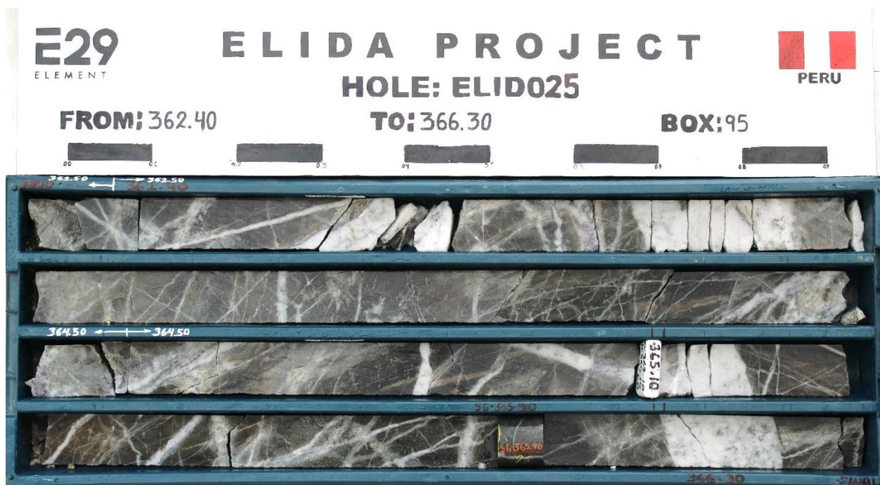
**Figure 11-3: The same interval shown in Figure 11-2 taken after sampling. Note the 5cm long cylinder of uncut core in the bottom row was preserved for specific gravity measurement. Source: Element 29 (2022).**
