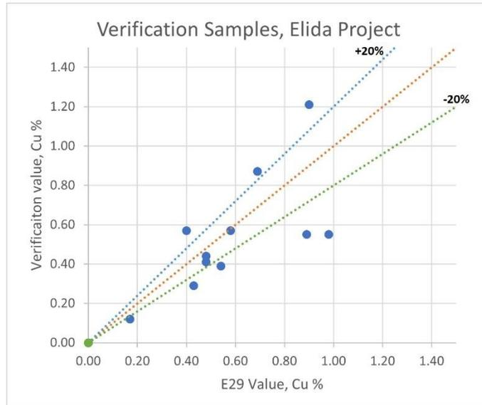
**Figure 12-18: Scatterplot of Cu values from replicate samples and corresponding values reported by Element 29.** Source Element 29 (2022).
