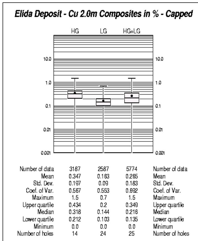
**Figure 14-11: Boxplots of composited and capped copper grades by domain, Elida deposit.** Source: Ginto (2022).
