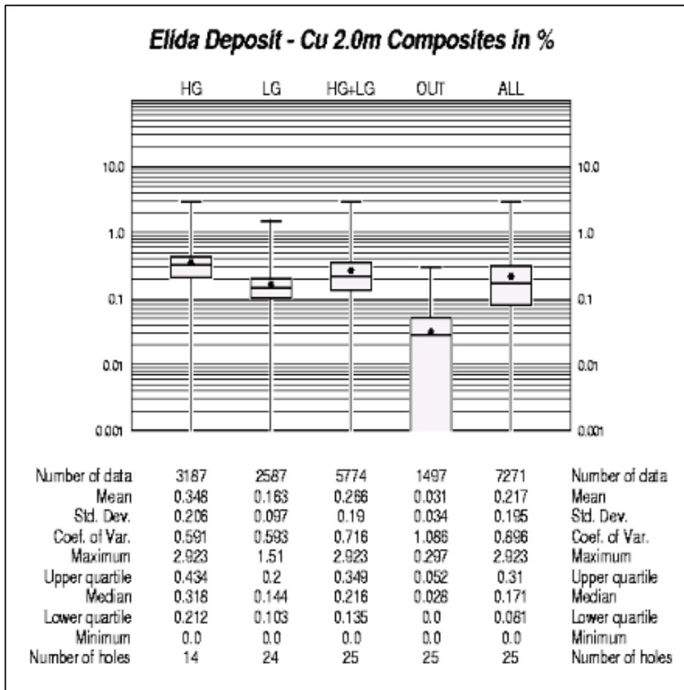
**Figure 14-8: Boxplots of composited copper grades by domain, Elida deposit.** Source: Ginto (2022).
