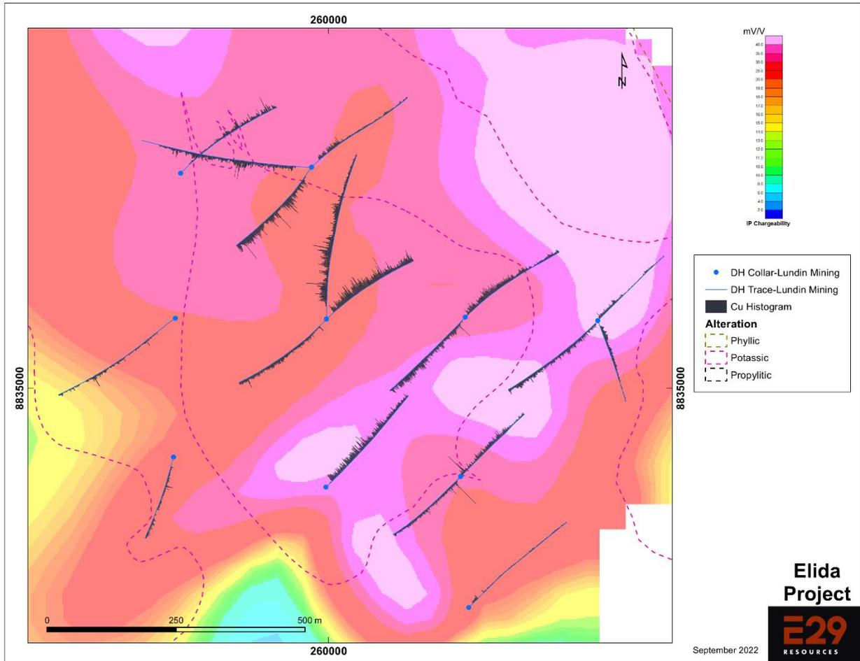
**Figure 6-2. Drill holes completed by Lundin in relation to chargeability at 1412 m elevation.**
