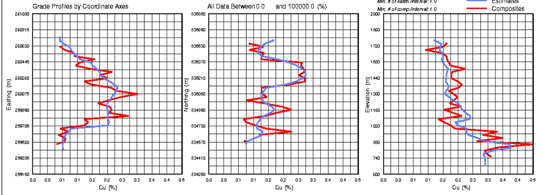
Figure 14-17: Copper grade profiles of declustered composites and block estimates, Elida deposit. Source: Ginto (2022).
