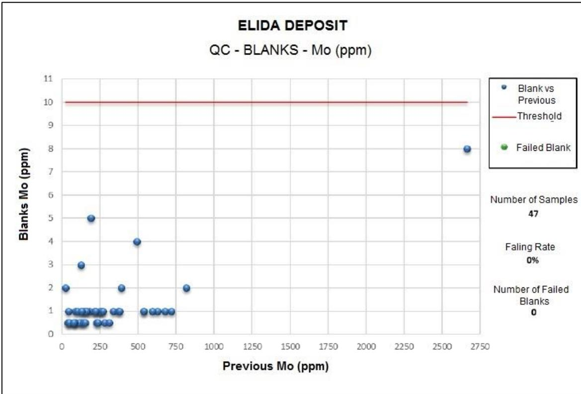
Figure 12-5:Dispersion of blanks for molybdenum, Elida project. Source: Element 29 (2022).
