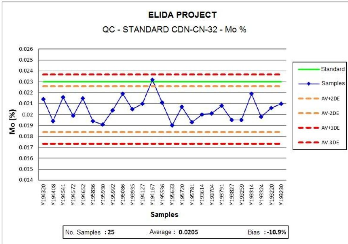
**Figure 12-8: Standard CDN-CM-32 for molybdenum, Elida project.** Source: Element 29 (2022).
