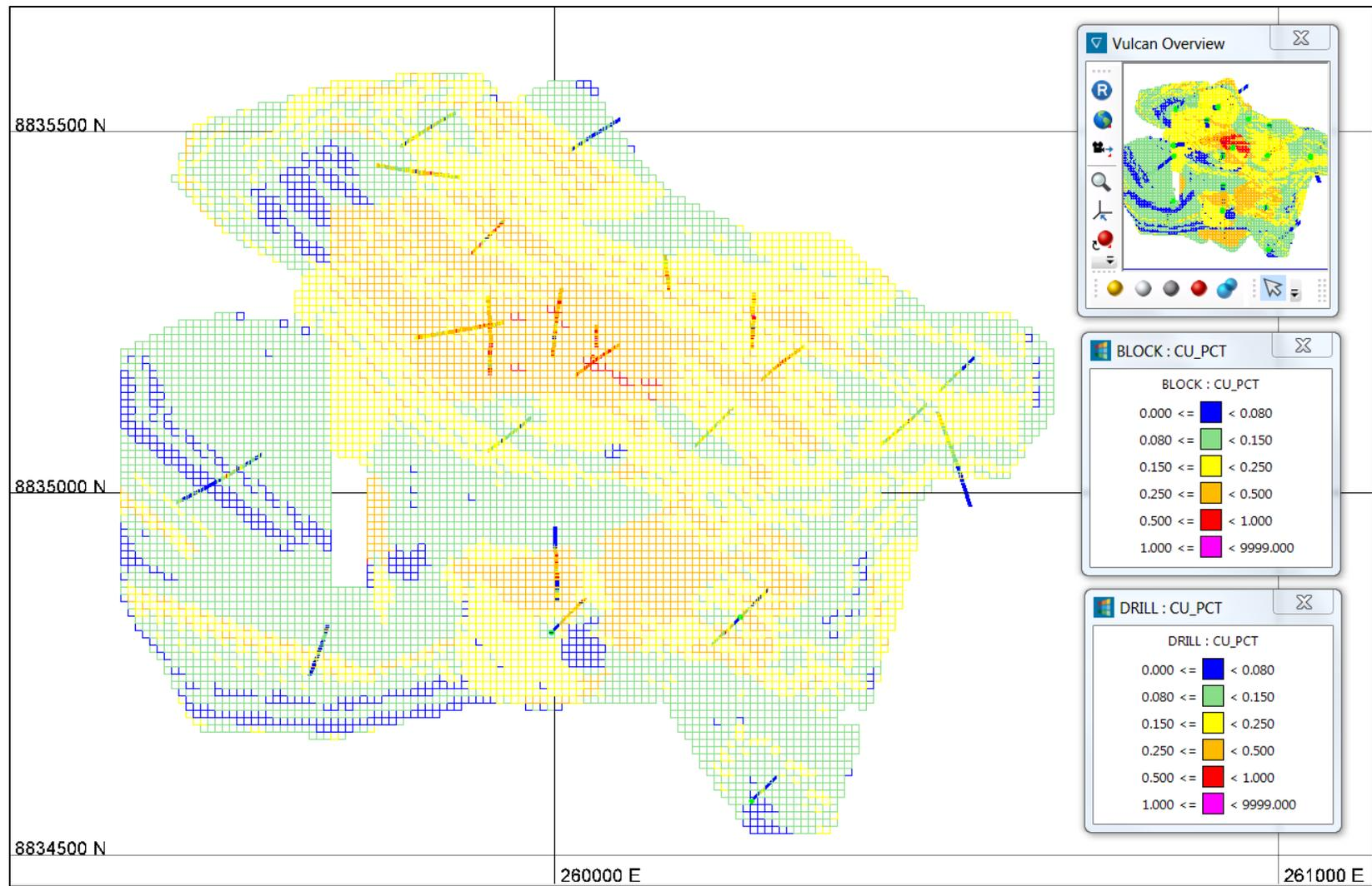
Figure 14-16: Copper block grade estimates and drill hole grades, level 1500 m. Elida deposit. Source: Ginto (2022).
