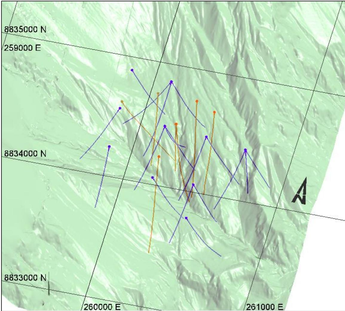
Figure 14-2: Drill hole location with topography. Perspective view looking northwest, Elida project. Lundin holes in blue, Element 29 holes in orange. Source: Ginto (2022).
