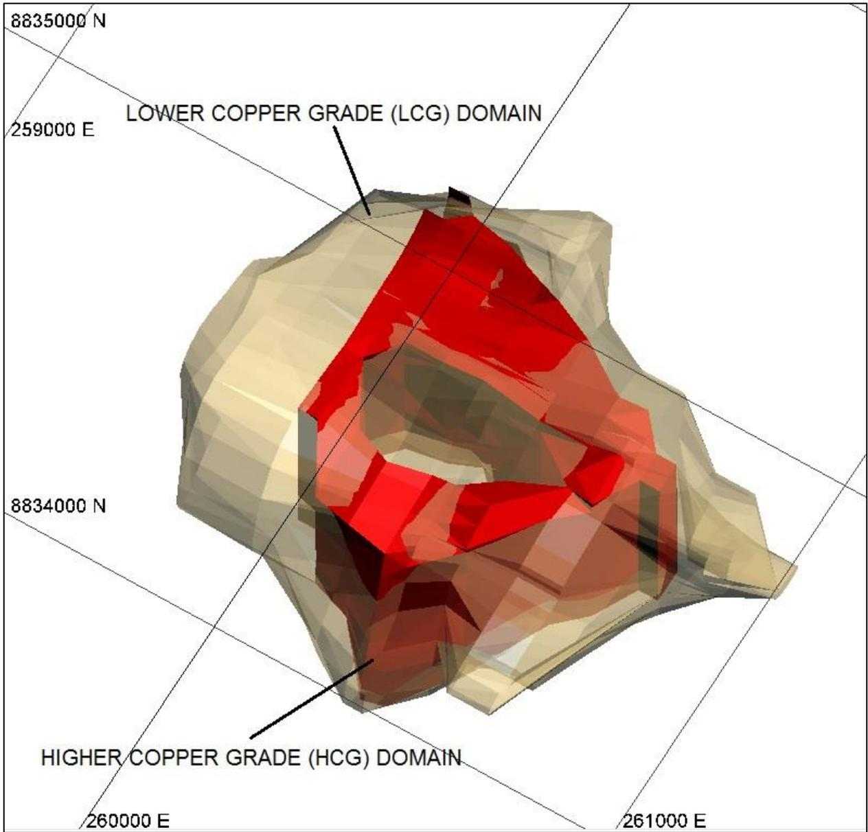
**Figure 14-4: Geology model, perspective view looking northwest. Elida deposit. Source: Ginto (2022).**
