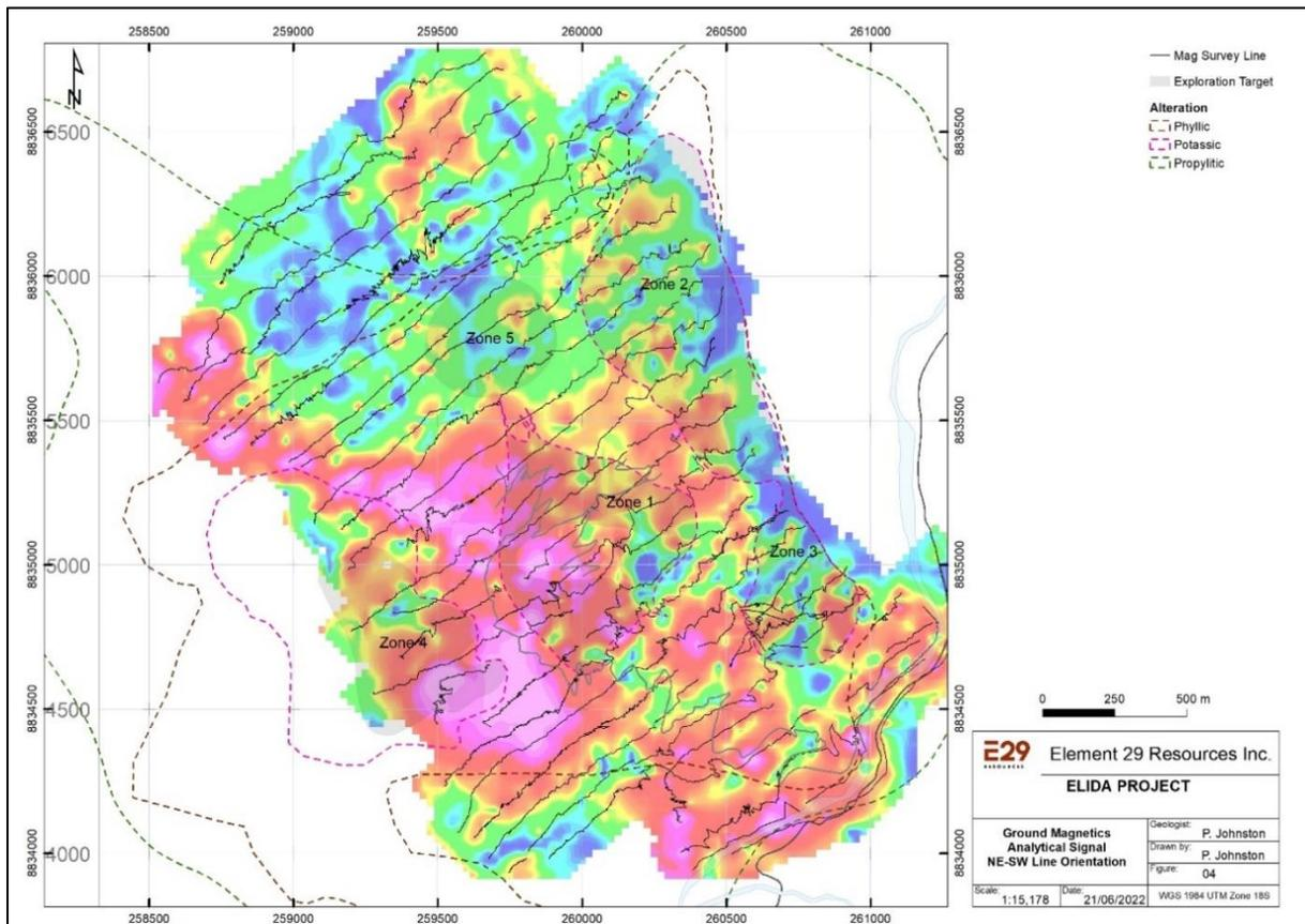
**Figure 6-3: Analytical signal from ground magnetic survey completed by Lundin in 2015 in relation to main alteration facies interpreted by Element 29 staff. Source: Element 29 (2022).**
