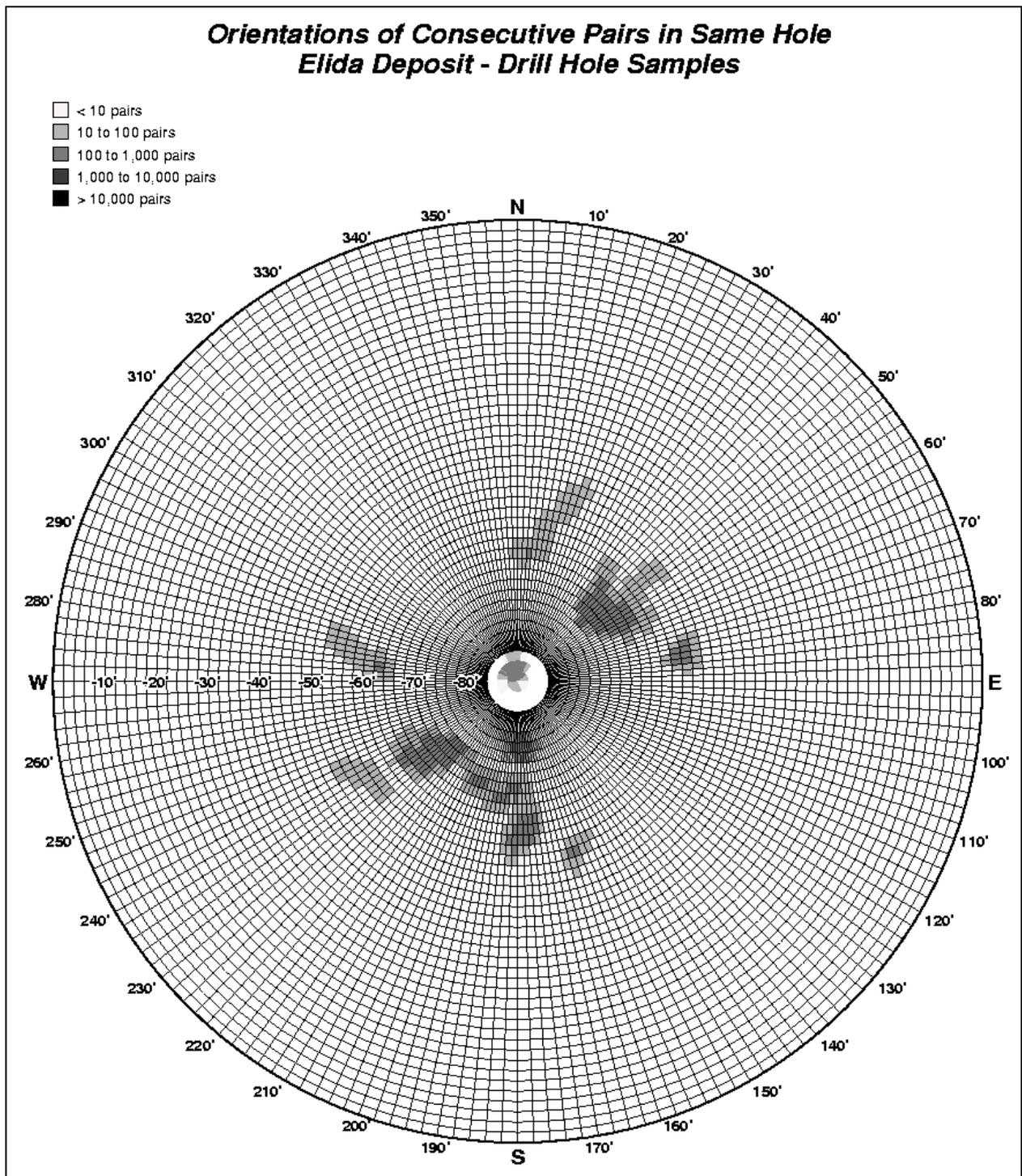
**Figure 14-7: Orientations and dips of drill holes, Elida deposit.** Source: Ginto (2022).
