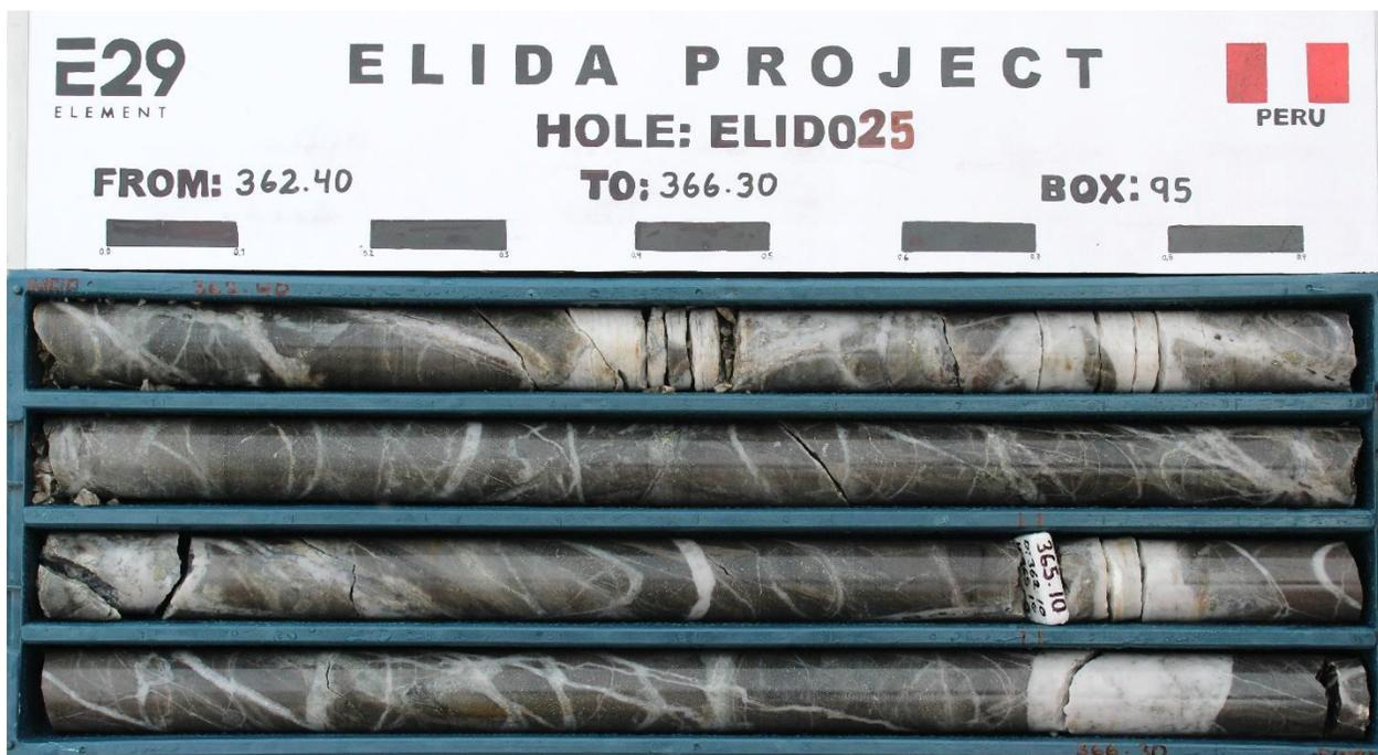
Figure 11-2: Example of a core photograph taken before sampling. Hole number, box number, and depth in metres are recorded on a standard panel with scale. Source: Element 29 (2022).
