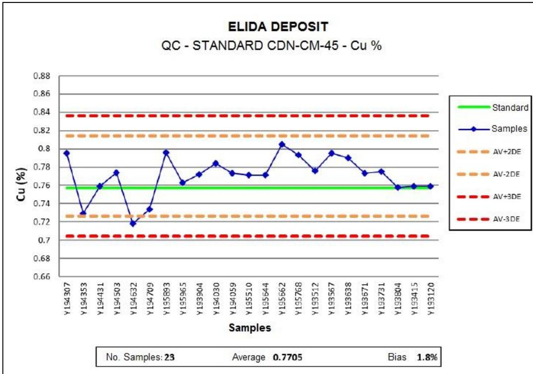
Figure 12-13: Standard CDN-CM-45 for copper, Elida Project. Source: Element 29 (2022).
