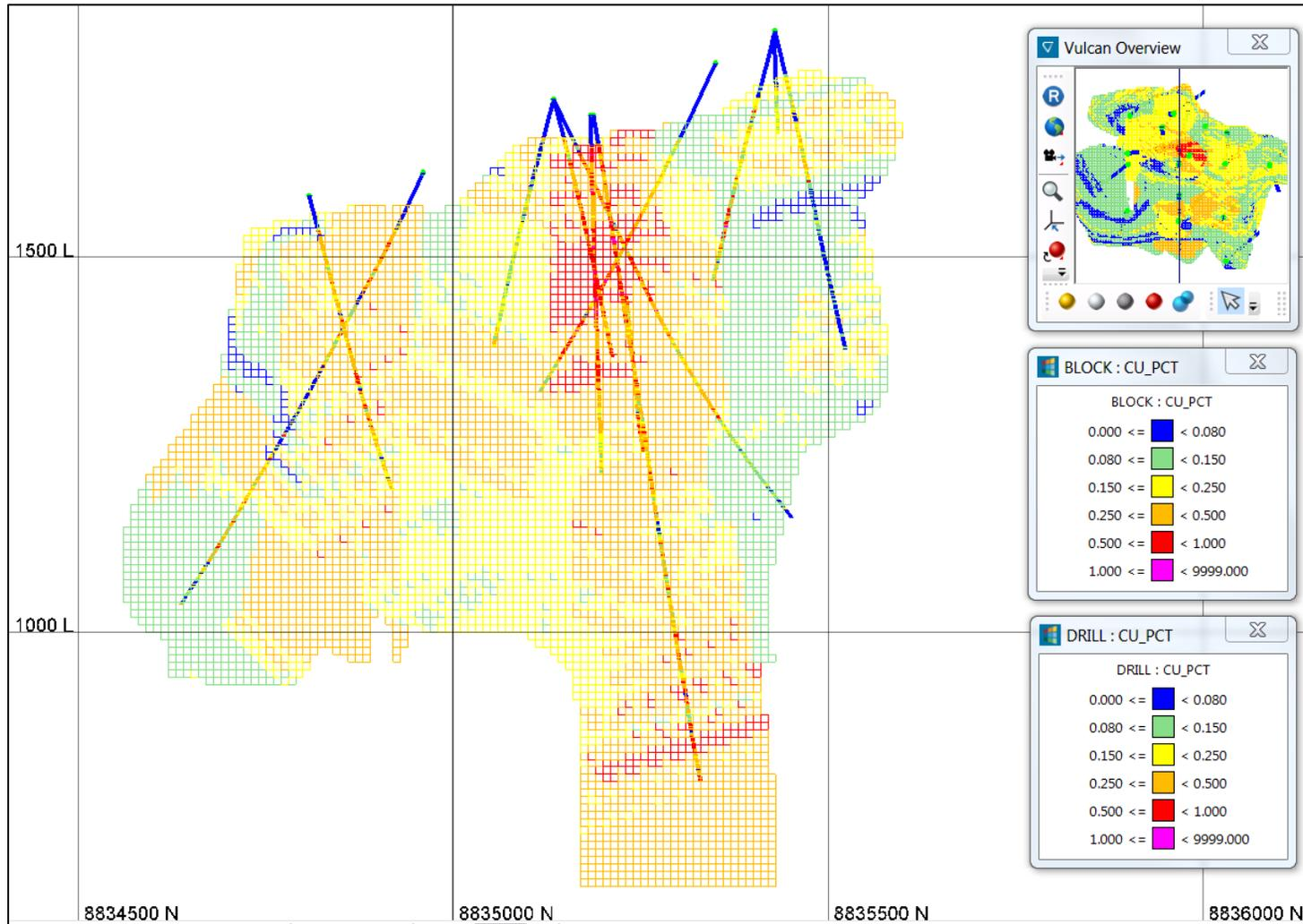
Figure 14-14: Copper block grade estimates and drill hole grades, Section 260,000E looking west. Elida deposit. Source: Ginto (2022).
