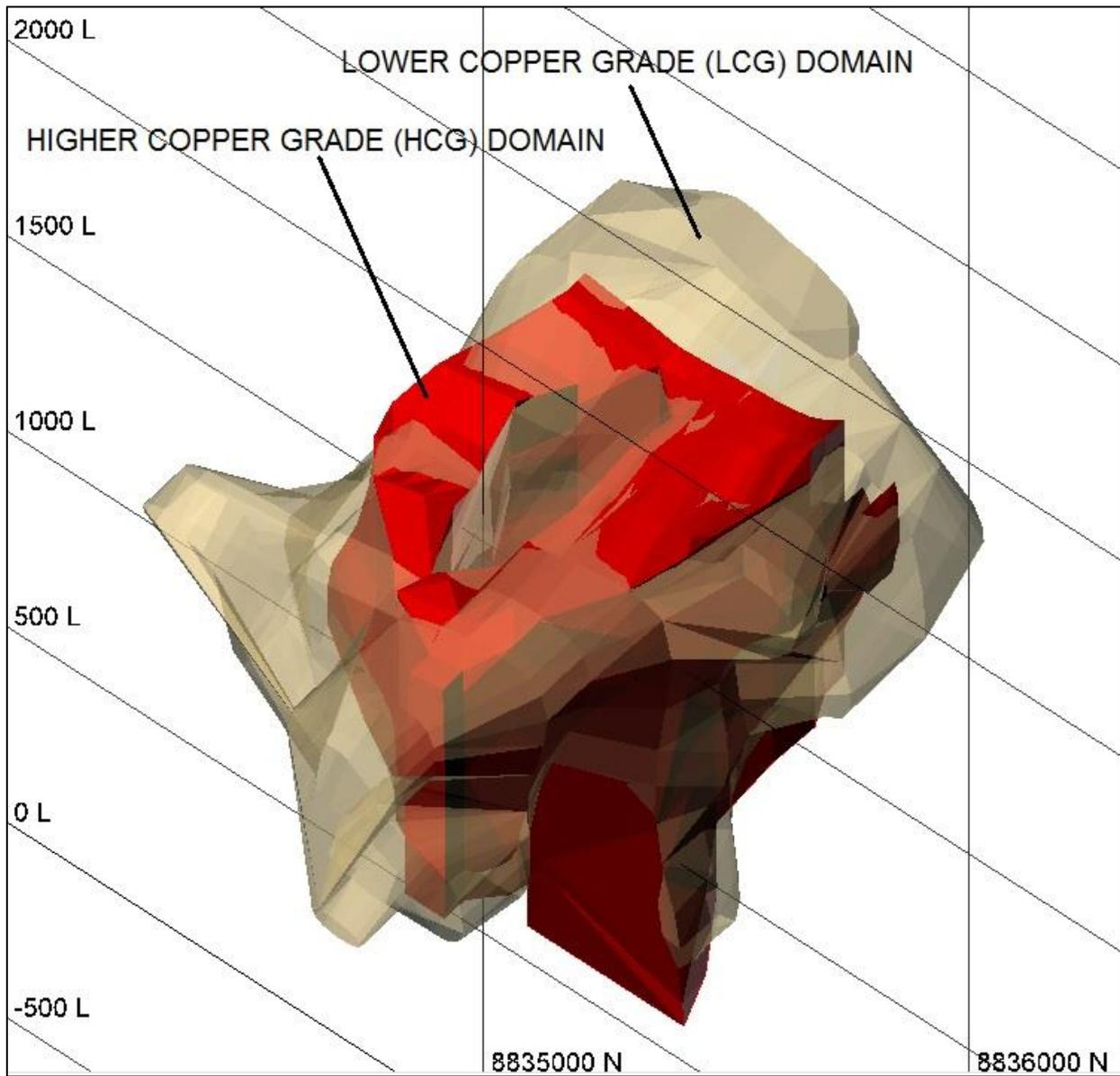
**Figure 14-5: Geology model, perspective view looking southwest. Elida deposit. Source: Ginto (2022).**
