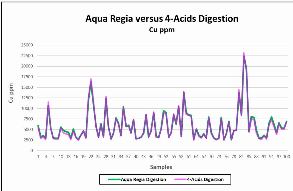
**Figure 11-8: Cu assay comparison of aqua regia and four-acid digestions from the Elida project 2021 drilling campaign.** Source: Element 29 (2022).
