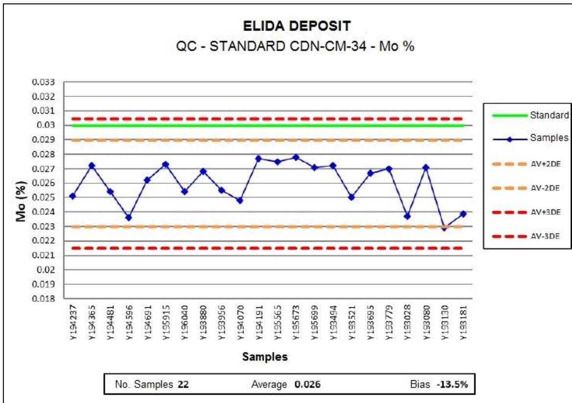
Figure 12-12: Standard CDN-CM-34 for molybdenum, Elida project. Source: Element 29 (2022).
