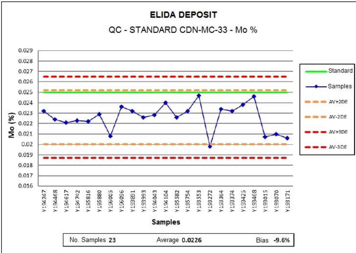
Figure 12-10: Standard CDN-CM-33 for molybdenum, Elida Project. Source: Element 29 (2022).
