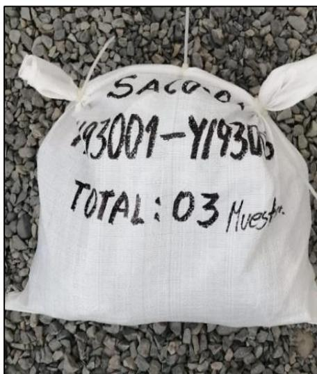
**Figure 11-6: Plastic-weave sacks used for shipping samples batches from the Elida project to the laboratory.** Source: Element 29 (2022).
