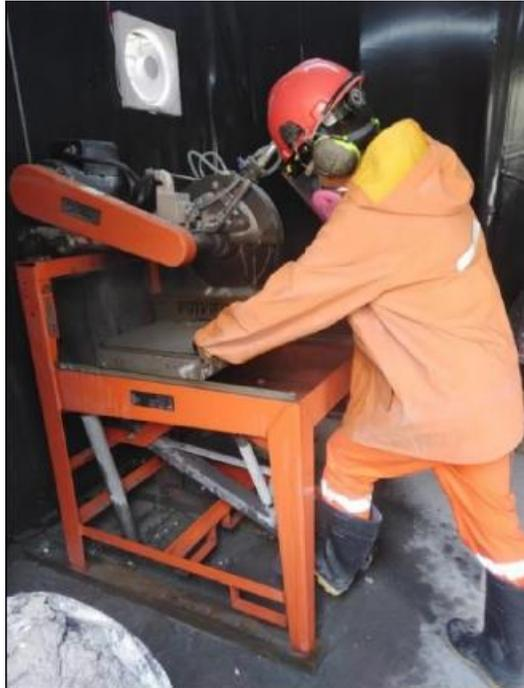
**Figure 11-4: Drill core cutting during the Elida 2021 drilling campaign using a rotary diamond blade saw.** Source: Element 29 (2022).
