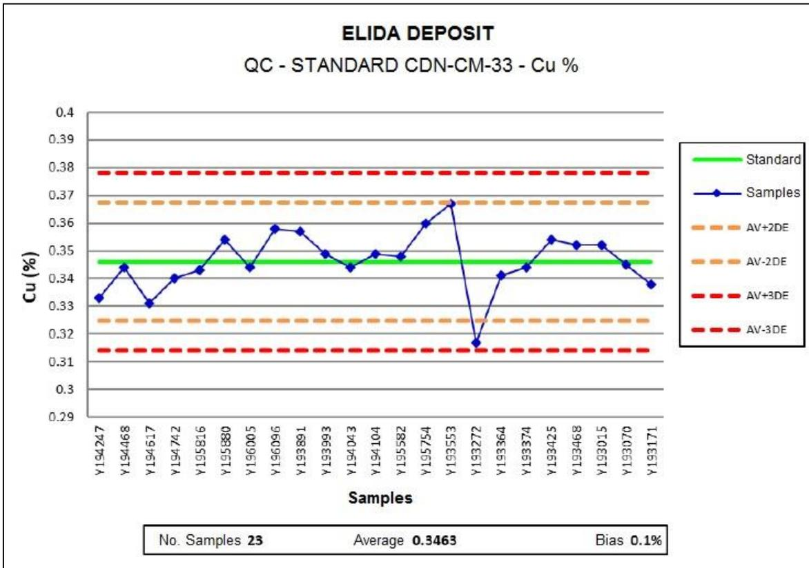
Figure 12-9: Standard CDN-CM-33 for copper, Elida Project. Source: Element 29 (2022).
