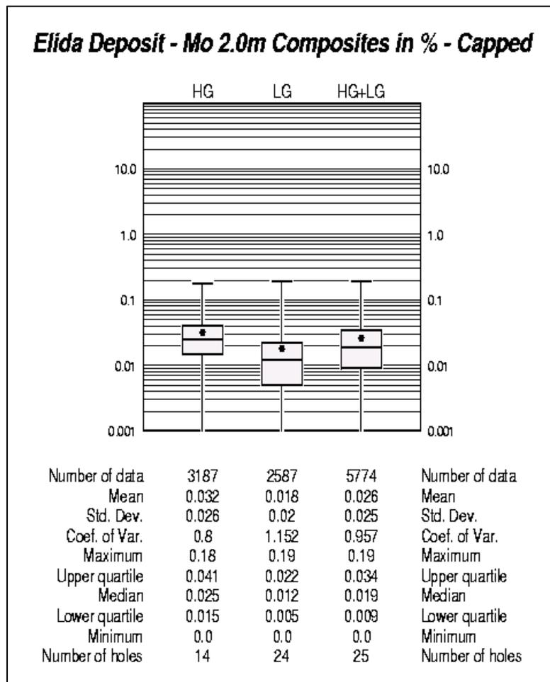
**Figure 14-12: Boxplots of composited and capped molybdenum grades by domain, Elida deposit.**
