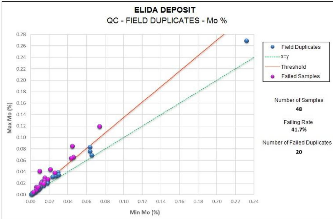
**Figure 12-2: Dispersion of field duplicates for molybdenum, Elida deposit.** Source: Element 29 (2022).
