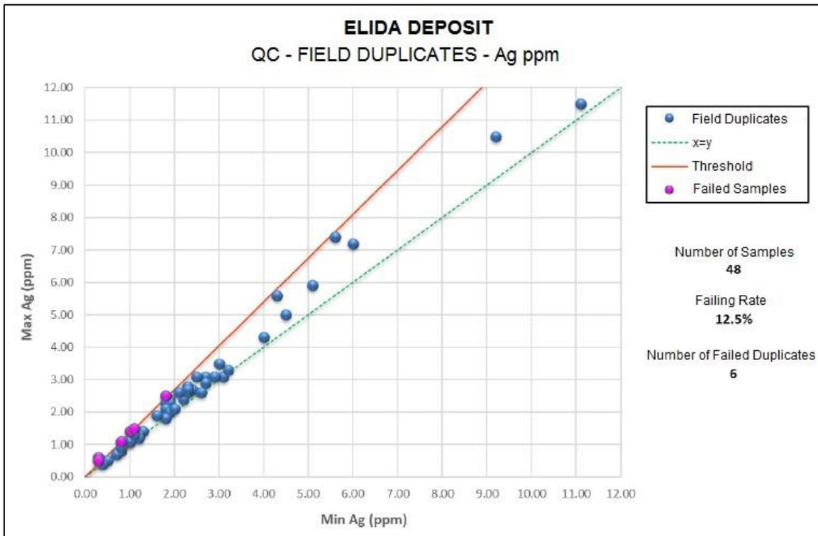
Figure 12-3: Dispersion of field duplicates for silver, Elida deposit. Source: Element 29 (2022).
