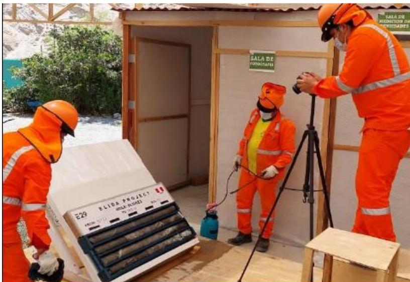
Figure 11-1: Core photography during the Elida project 2021 drilling campaign. Source: Element 29 (2022).
