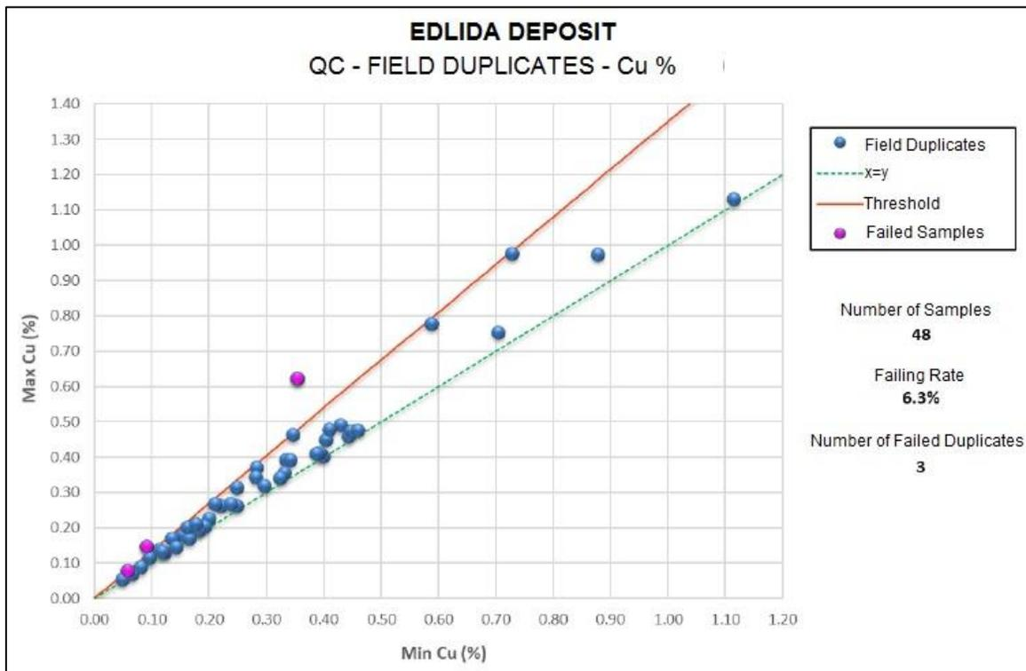
**Figure 12-1: Dispersion of field duplicates for copper, Elida deposit.** Source: Element 29 (2022).
