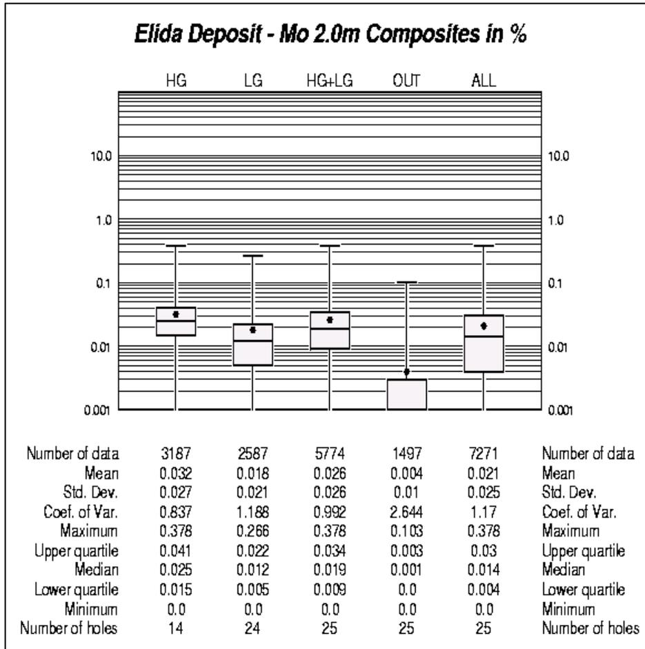
**Figure 14-9: Boxplots of composited molybdenum grades by domain, Elida deposit.** Source: Ginto (2022).
