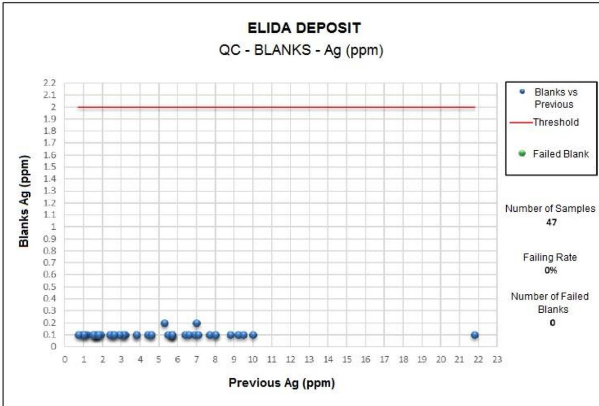
Figure 12-6: Dispersion of blanks for silver, Elida project. Source: Element 29 (2022).
