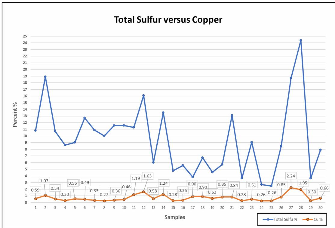
**Figure 11-11: Total sulfur assays by LECO compared with Cu assays from the Elida project 2021 drilling campaign.** Source: Element 29 (2020)
