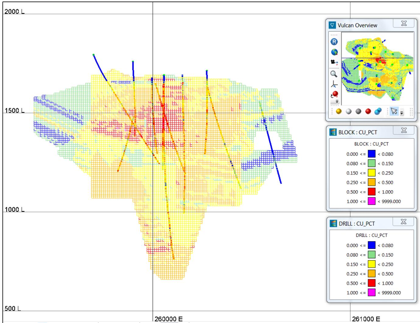
Figure 14-15: Copper block grade estimates and drill hole grades, Section 8,835,250N looking north. Elida deposit. Source: Ginto (2022).
