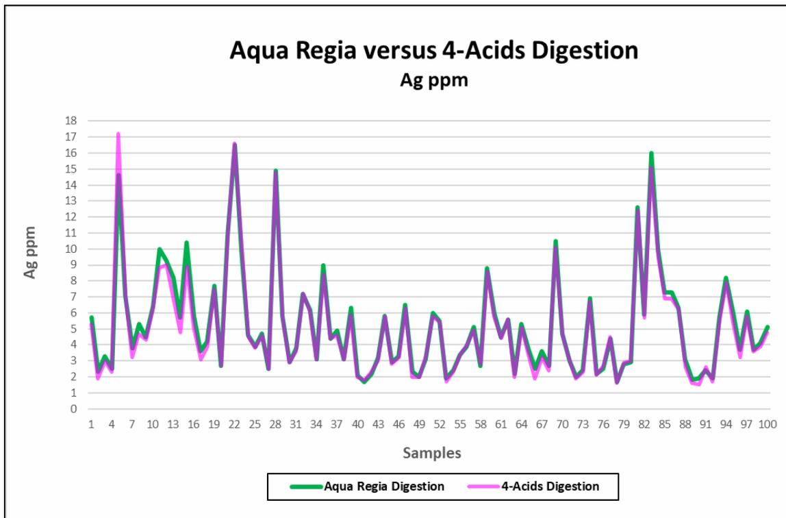
Figure 11-10: Ag assay comparison of aqua regia and four-acid digestions from the Elida project 2021 drilling campaign. Source: Element 29 (2022).
