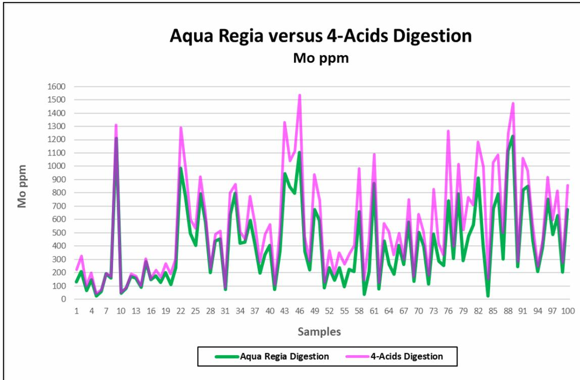
Figure 11-9: Mo assay comparison of aqua regia and four-acid digestions from the Elida project 2021 drilling campaign. Source: Element 29 (2022).
