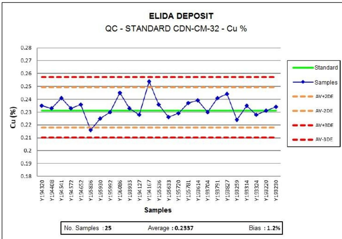
**Figure 12-7: Standard CDN-CM-32 for copper, Elida project.** Source: Element 29 (2022).
