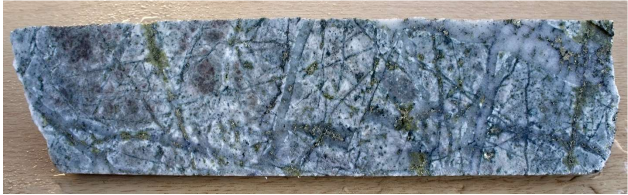
Figure 13. ELID019, 241.15m from a sample interval reporting 0.62% Cu, 0.032% Mo, 4.4 g/t Ag . Intense, multiple generations of A-type veins in feldspathic arenite host rock. The A-type veins contain an assemblage of pyrite-chalcopyrite-molybdenite with minor magnetite. Chalcopyrite is also introduced by green mica veinlets containing chlorite, epidote with chalcopyrite and pyrite. Core is HQ diameter (63.5 mm).
