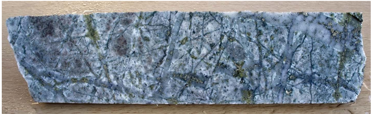
Figure 17. ELID019, 241.15m from a sample interval reporting 0.62% Cu, 0.032% Mo, 4.4 g/t Ag. Intense, multiple generations of A-type veins in feldspathic arenite host rock. The A-type veins contain an assemblage of pyrite-chalcopyrite-molybdenite with minor magnetite. Chalcopyrite is also introduced by green mica veinlets containing chlorite, epidote with chalcopyrite and pyrite. Core is HQ diameter (63.5 mm).
