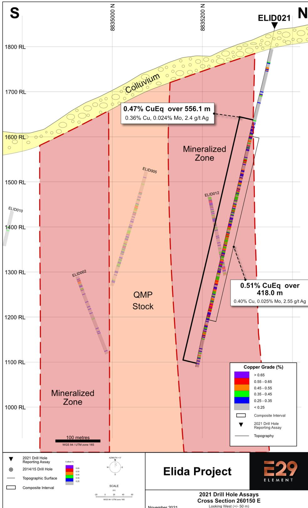
**Figure 3.** Cross section 260250 E showing hole ELID022. The hole entered anomalous Cu mineralization associated with weak potassic alteration beneath approximately 35 m of unconsolidated colluvial gravel. The hole was designed to constrain the near-surface northern limit of mineralization, obtain information on the northern part of the mineralized zone, and confirm the eastward continuity of mineralization intersected by ELID021.
