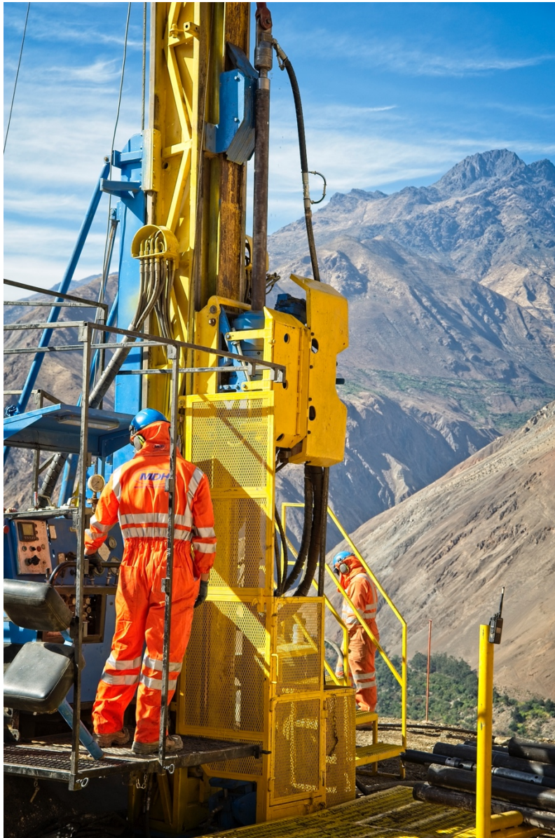
Figure 11. Drilling unit initiating drilling of hole ELID019. Drilling equipment is configured to drill a vertical hole up to a depth of 1,000 metres.
